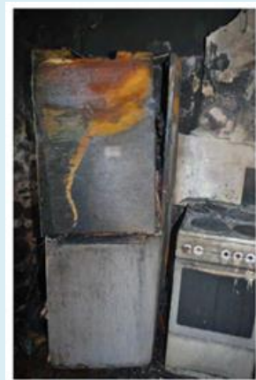
Refrigerator that started the fire [2]
